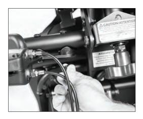
**29A.** Run the cables inside the adjustment wheel. Insert tie strap into hole
