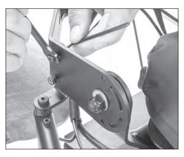
**20.** Insert 2 bolts and 2 nuts and tighten securely.
