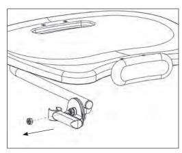
**32.** If the swing away shadow tray was ordered, using a wrench, remove the nut from the bolt on the tray arm and discard the nut. Make sure all other hardware stays on the bolt.
