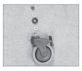
2. Remove the hardware on both casters and set out as shown. This is how the hardware will be assembled. The casters are supplied with a locking compound pre-applied to the threaded stem. Do not remove this material, it is important to prevent the casters from loosening over time. Make sure the caster is in the lock position as shown.
