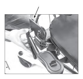
**19.** Place controler bracket onto the inside of the hip pivot bracket as shown
