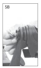
**6.** Making sure the caster is in the locked position, place the lock nut onto the caster stud and tighten securely using provided wrench.
