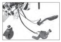
**9A.** Remove the screw from the following arm and set the screw aside. You will need this later.
