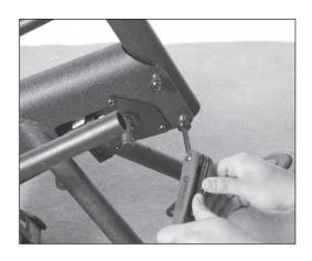
25. While supporting the front wheel assembly, using the 4 bolts and lock washers that were removed from the front wheel assembly, insert and start the 2 top bolts into the base and wheel assembly, than insert and start the 2 lower bolts, making sure to start all 4 bolts before tightening securely.
