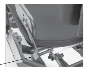
**39.** If the Hip Supports were ordered, loosen knob on tube on the back rear of the seat. Insert bracket into the tube and tighten securely.
