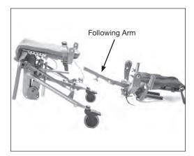
**8.** With assistance, place the base unit as shown, if the back option was **NOT** ordered, skip to step #21. Place the back as shown and place the following arm as shown.
