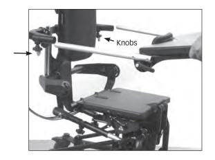
**31.** Lock the casters, loosen the knobs on the tray receiver all the way, then flip open gray tabs until it clicks. Insert the two tray arms into the tray bracket on the bottom of the tray as shown.
