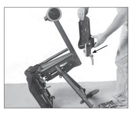
**26.** Loosen ratchet handle and place both foot plates on the unit, with the ratchet handle to the outside of the unit.
