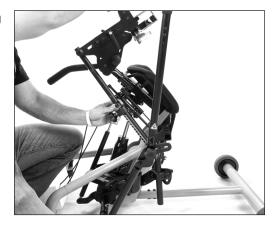
**10.** Depress the spring button to allow the following arm to slide into place. Match the following arm position color with the corresponding seat depth color. Tighten the knob securely (for information on seat adjustments see the Instructions for Use Manual).
