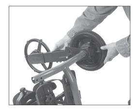
**31.** Line up the holes and tap in the coved nuts and tighten bolts securely. Making sure the coved nuts are flush with the base. Position the Bantam upright and re-tighten the frame bolts.
