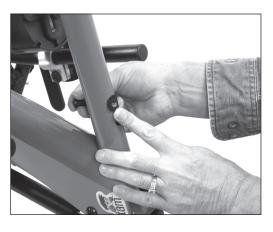
**30.** Attach the interchangeable right and left drive wheel assemblies to the front frame.
