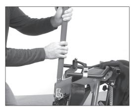
**3.** Place the two coved nuts into the bottom of the frame and flush with the tube. You may have to tap them in with a rubber hammer to make them flush.
