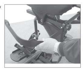
14. Remove knob from the knee pad, leaving the plastic and rubber washer in place on the knee pad, place the knee pad and washers onto the knee pad bracket. Place knob onto bolt as shown. Repeat steps for the opposite side (for information on knee pad adjustments see the Instructions for Use Manual).
