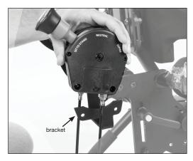
**17.** Making sure the nuts are in the back on the controller, line up holes and insert both bolts. Tighten securely.
