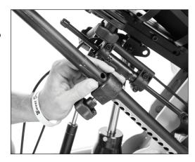
**11.** Loosen the ratchet handles on the foot plates and swivel into place (for information on foot plate adjustments see the Instructions for Use Manual).
