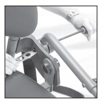
4. Place lock washer and nut onto bolt. Using a hex tool and wrench tighten securely.
